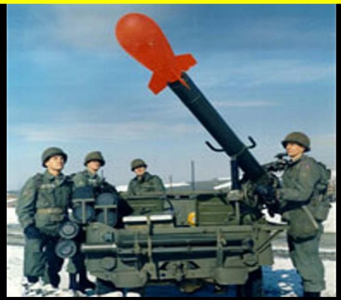
W-54 DAVEY CROCKETT WARHEAD ON A RECOIL-LESS RIFLE PU-239 CORE 22 TONS TO 1 KT RANGE 2.5 MILES
